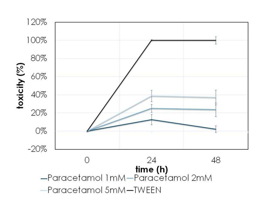
Increasing concentrations of paracetamol induce a decrease in base impedance of monocyte-derived hepatocyte-like (MH) cells which can be monitored continuously (left). Tween (2%) induced 100% cell death and was used as a positive control. The data is compared with the toxicity measurement of MH cells using an LDH release assay (right).
