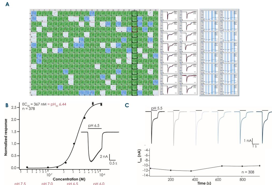
**Figure 2: Activation of ASIC1a on the SyncroPatch 384i.** A: Screenshot depicts raw data traces of ASIC1a-expressing CHO cells as recorded on one NPC-384 patch clamp chip (single hole per well). Solution at pH 6.5 was applied to the cells (exposure time 1 s) and then washed away by control solution [pH 7.2]. B: pH response curve for an average of 378 wells revealed a  $pH_{0.5} = 6.44$  in excellent agreement with literature values<sup>2,3</sup>.
