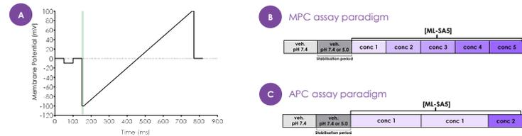
**Figure 1.** Currents were elicited using the voltage protocol shown in (A), applied at 0.1 Hz, with peak inward current amplitudes measured at -100 mV (indicated by green cursor). Assay paradigms used in the manual patch-clamp assay are depicted in (B). Assay paradigms used for the automated patch-clamp assay are shown in (C). For both MPC and APC, whole-cell conformation is obtained in pH 7.4. Inward currents were stabilised in either pH 7.4 or 5.0.
